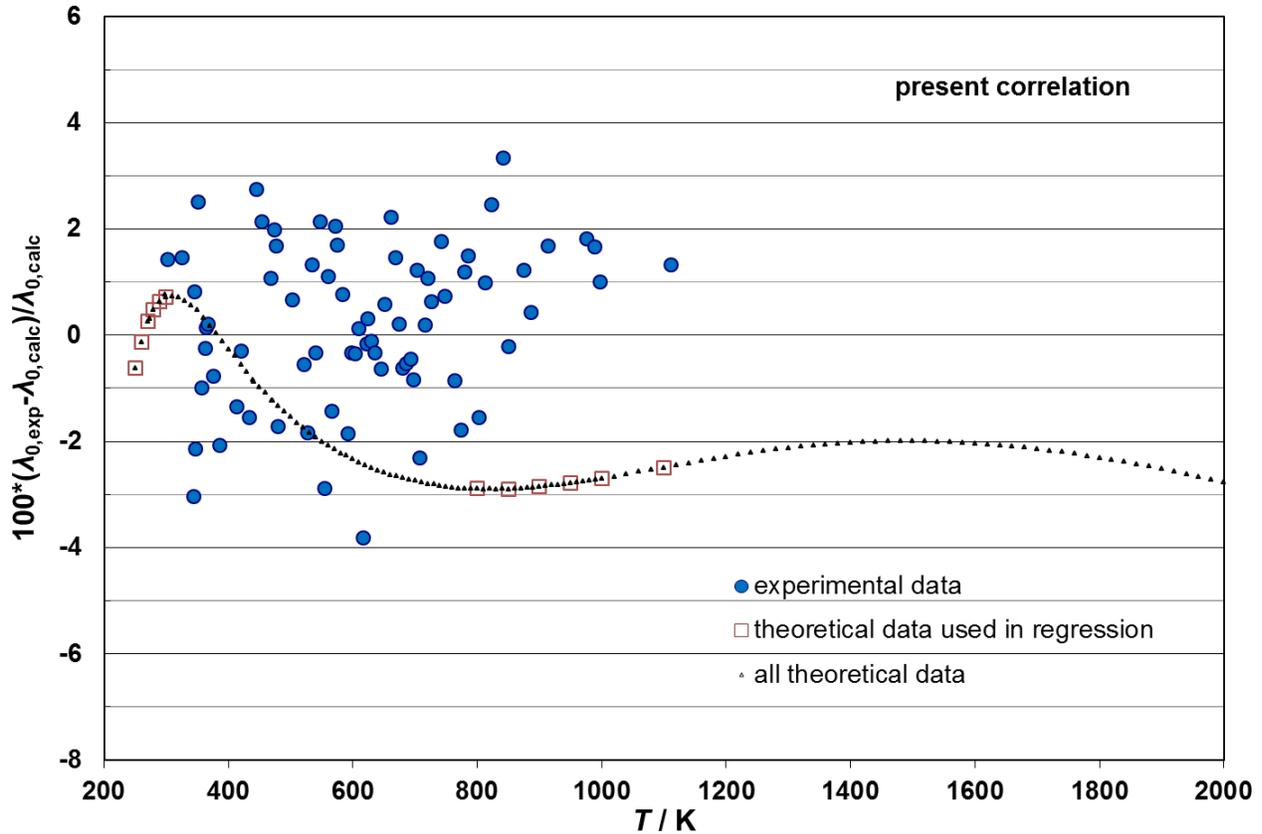
Figure 1. Percent deviation of experimental low-density thermal conductivity data and values calculated from theory [7] from IAPWS formulation for thermal conductivity [4,5]. Figure from Ref. [5]
